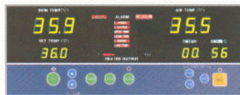
Computerized control system integrates all necessary controls, indicators, displays and alarms in a single location
